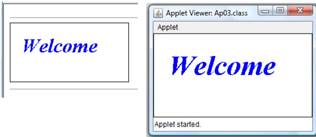
As Applet Viewer allows us to change the display area's size, we can test our applet to make sure it is not dependent on absolute sizes and/or coordinates. (By the way, we can change our display area's size explicitly from within an applet by calling `Applet.resize`.)
