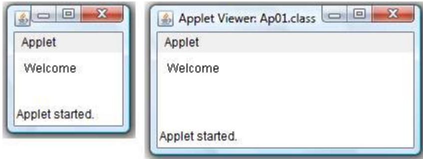
Unlike the browsers, Applet Viewer allows the size of its display specified by the HTML file to be overridden. As we can see in the right-hand picture above, the width and height have been increased. We'll exploit this feature of Applet Viewer in future examples.
